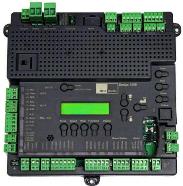
1050US Control Board
