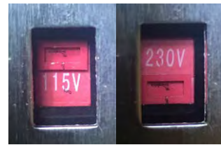
Figure 19. Voltage Switch Positions
