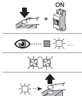
**(\*3) Note** - If the LED emits a steady red light, it means that the memorisation procedure was not completed. In this case, repeat the procedure from the beginning.
