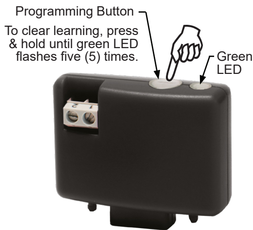
Fig-1: Radio Receiver Module OXIBD/A
