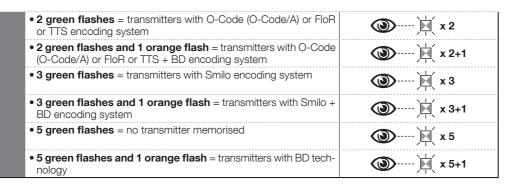
To change the coding assigned to the <u>first one-way transmitter memorised</u>, it is necessary to delete from the memory <u>all the transmitters present (one-way and two-way</u>), by strictly adopting Procedure 5 (Paragraph 3.6) and choosing the option, "ALL THE RECEIVER MEMORY".
