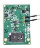
The 2GIG-LTEV1-NET-GC2 is a 4G LTE radio for the Verizon network to work with SecureNet. This new radio transfers both data and two-way voice over Verizon's 100% LTE network and VoLTE (Voice over LTE) technology.
