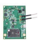
The 2GIG-LTEV1-A-GC2 is a 4G LTE radio for the Verizon network to work with Alarm.com. This new radio transfers both data and two-way voice over Verizon's 100% LTE network and VoLTE (Voice over LTE) technology.
